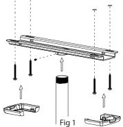
c. Thread in extension pipe and tighten set screws provided.
