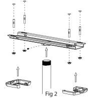
c. Re-install washer and bolt onto end of bolt and tighten down using a 7/16" socket head wrench until secure (per instructions with wall anchor).
